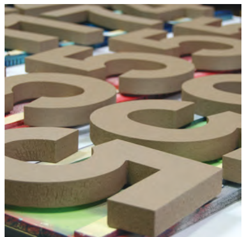
Foam numbers Router Cut and then lightly sanded and painted
