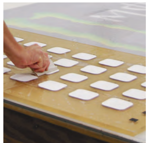
Sub-surface vinyl on clear acrylic applied by wet application
