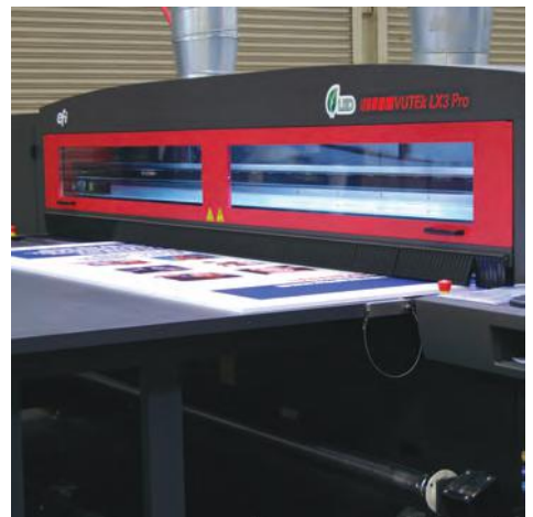
48" x 96" sheets of Gator Foam with direct print.
