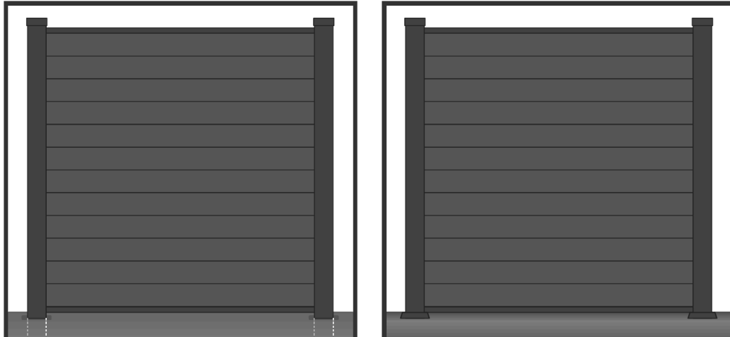
FIG. 1 – INSTALLATION OPTIONS – CONCRETE FOOTING (LEFT) AND PRE-PREPARED FOUNDATION (RIGHT)
