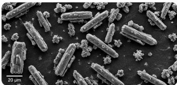
20 μm SEM image of HiCel™ SMCC (Silicified Microcrystalline Cellulose)
