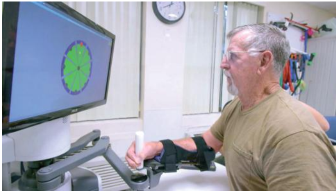
• Fig. 12.55 A 2-degrees of freedom robotic arm. The patient grips a handle at the end-effector and can push the handle in the horizontal plane, and two motors of the robot will drive the shoulder and elbow joints to follow. (InMotion2 courtesy Bionik Labs, Watertown, MA. https://bioniklabs.com/overview/ .)
