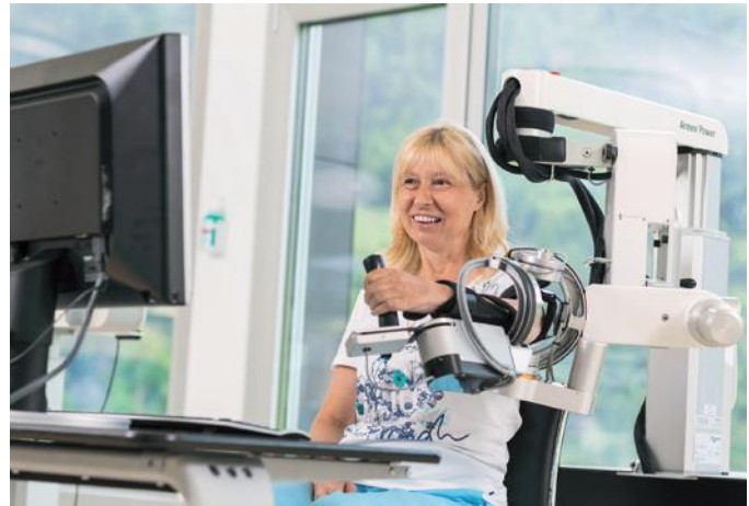
• Fig. 12.56 Up to 7-degrees of freedom robotic arm. A highly sensitive hand grip and videogame-like exercises to simulate arm movements used in specific real-life tasks through a virtual environment with immediate feedback. Armeo®Power image courtesy Hocoma (Volketswil, Switzerland).
