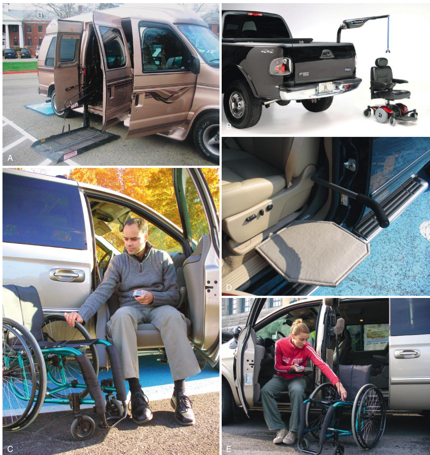
• Fig. 15.29 Vehicle lift systems. (A) Platform lift. (B) Overhead strap lift. (C) Automated height adjustable vehicle seat. (D) Automated height adjustable platform. (E) Side-door overhead wheelchair lift system. (B, Courtesy Braun Corp., Winamac, IN; C, courtesy St. Lambert, Quebec, Canada.)
