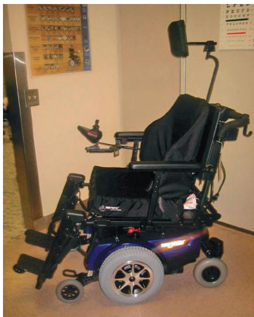
• Fig. 15.19 Indoor-outdoor power wheelchair shown with rehabilitation seating, a power tilt and recline seating system, head rest, and power-elevating leg rests.
