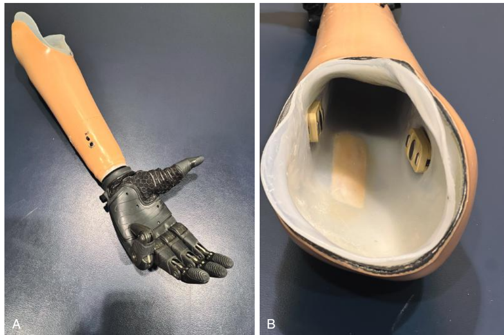
• Fig. 10.5 Myoelectric prosthesis (A) with myoelectric control system (B) for a transradial amputee with socket electrodes visible.
