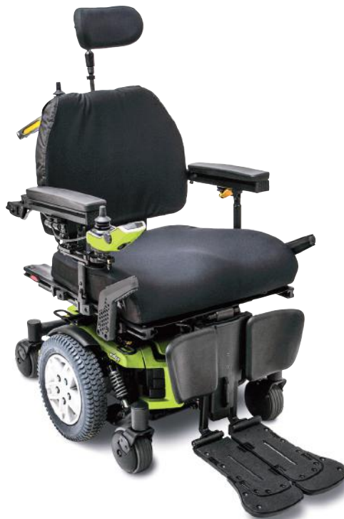
• Fig. 15.21 Heavy-duty indoor-outdoor power wheelchair. (Courtesy Quantum Rehab, Duryea, PA.)
