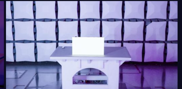
Anechoic Chamber RF Test
