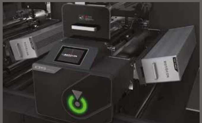
The multi-servo-driven flexo printing unit
