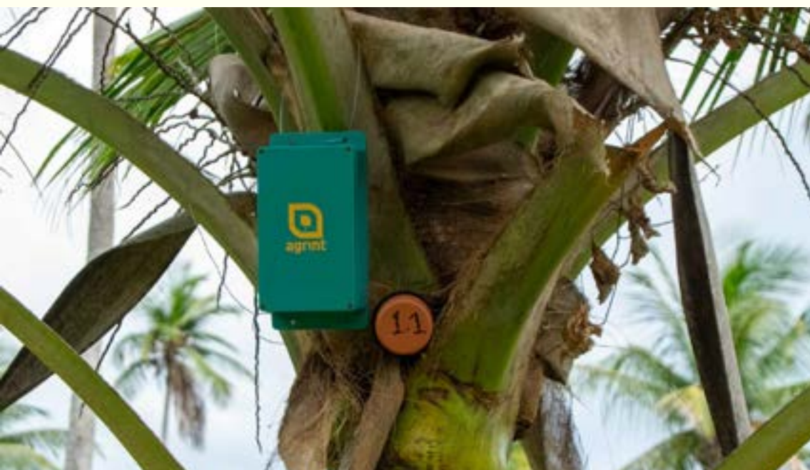
Photo: IoT Sensor to detect the presence of South American Palm Weevil larvae in coconut tree, Trinidad and Tobago. © N. Sharma/CARDI
