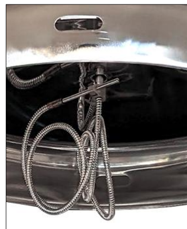
Load sensing probe stows away in lid when not used
