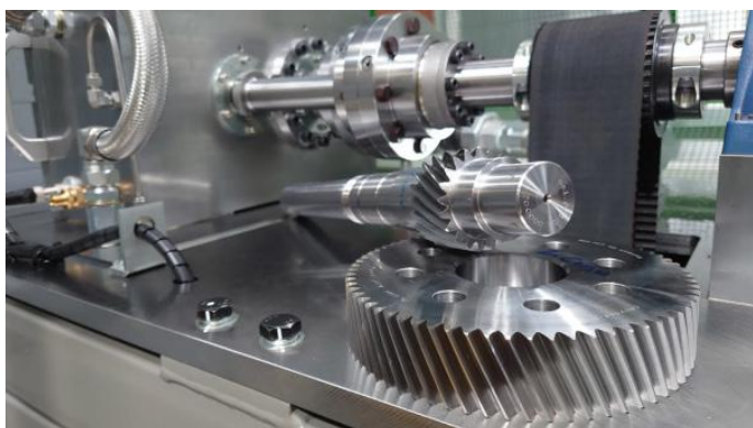
An in-house back-to-back rig built for non-involute gears. (All images: Dontyne)
