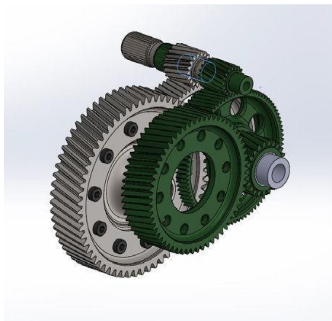
An in-house back-to-back rig built for non-involute gears. (All images: Dontyne)
