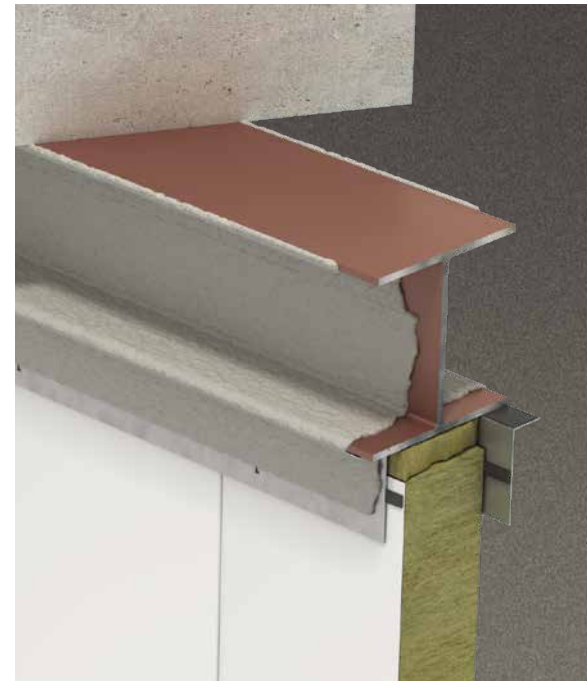
Spray protection to steel header
