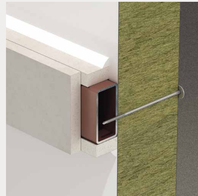
Optimised solution - K-Roc® Firemaster Wall Panel protects the connecting face
