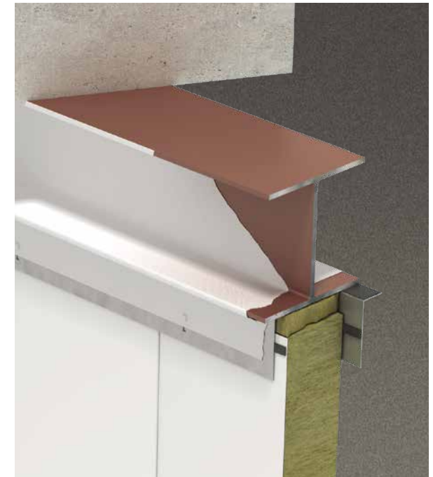
Intumescent coating protection to steel header
