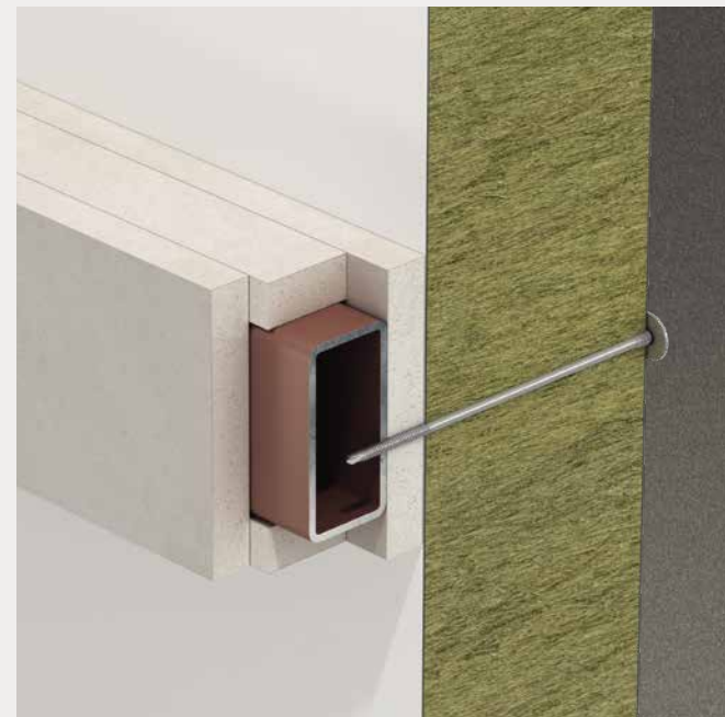
Traditional approach - steel member protected on all sides
