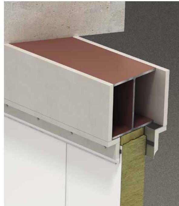
Board protection to steel header
