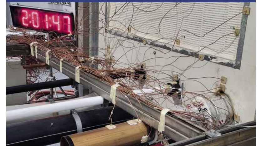
FIREFLY penetration solutions in K-Roc® Firemaster Wall Panels at 2 hours into an AS 1530.4: 2014 test
