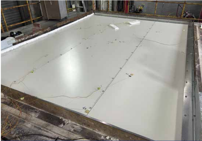
K-Roc® Firemaster Ultima Plus Ceiling Panels during AS 1530.4: 2014 fire test
