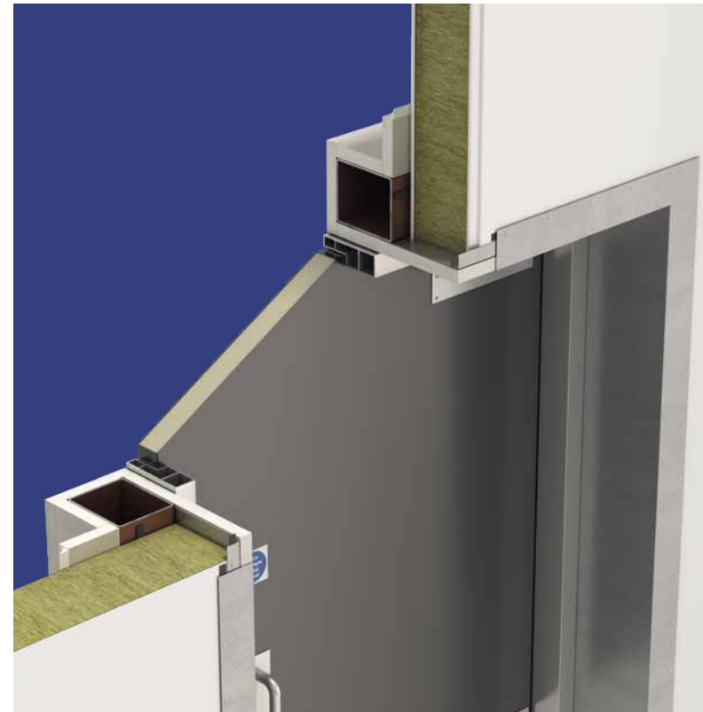
Out-of-plane double doorset with fire protected structural support
