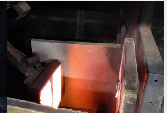
AS/NZS 1530.3: 1999 small-scale fire test for fire hazard properties (image courtesy of AWT Product Testing)
