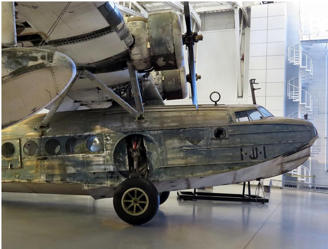
A close-up of the nose section of the Sikorsky JRS-1. This photo shows how the JRS-1's conventional landing gear retracted into the hull. This photo also shows how the JRS-1's engines were mounted on the wing above the hull. Sikorsky chose this engine layout to keep them free of sea spray when the aircraft was used as a flying boat. The Consolidated PBV Catalina flying boat, which saw service in World War II, had a similar layout for its engines.
