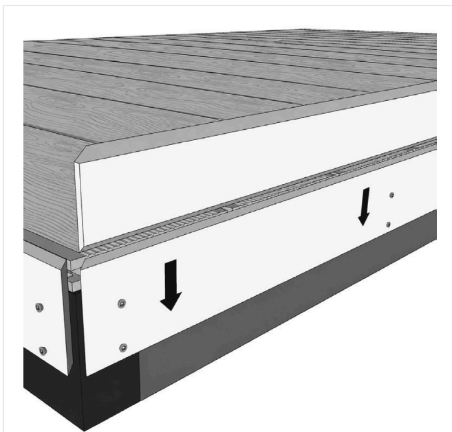
FIG. 25 - CORNER TRIM PLACED OVER THE DECK EDGE
