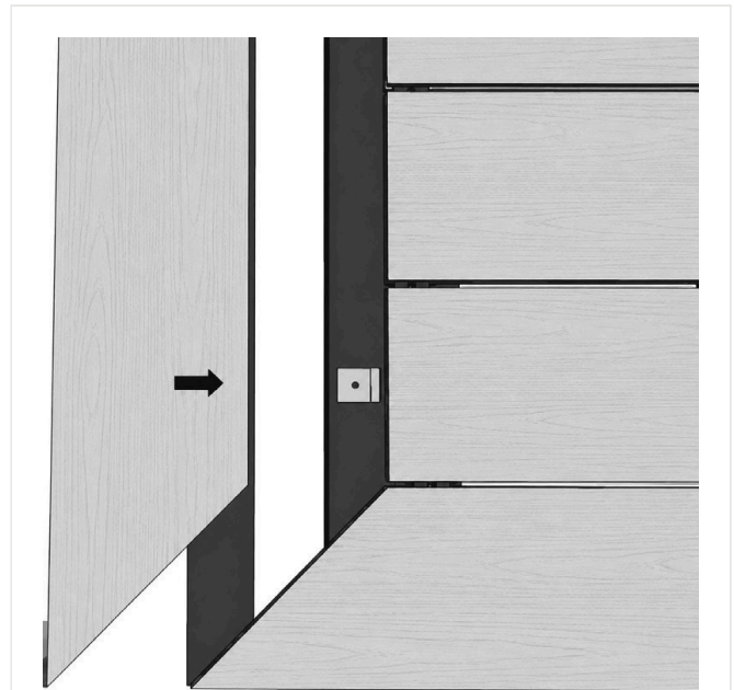
FIG. 15 – PICTURE-FRAME BOARD SLID INTO THE STARTER CLIPS
