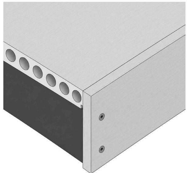
FIG. 24 – COUNTERSUNK PILOT HOLES PRE-DRILLED THROUGH THE FASCIA
