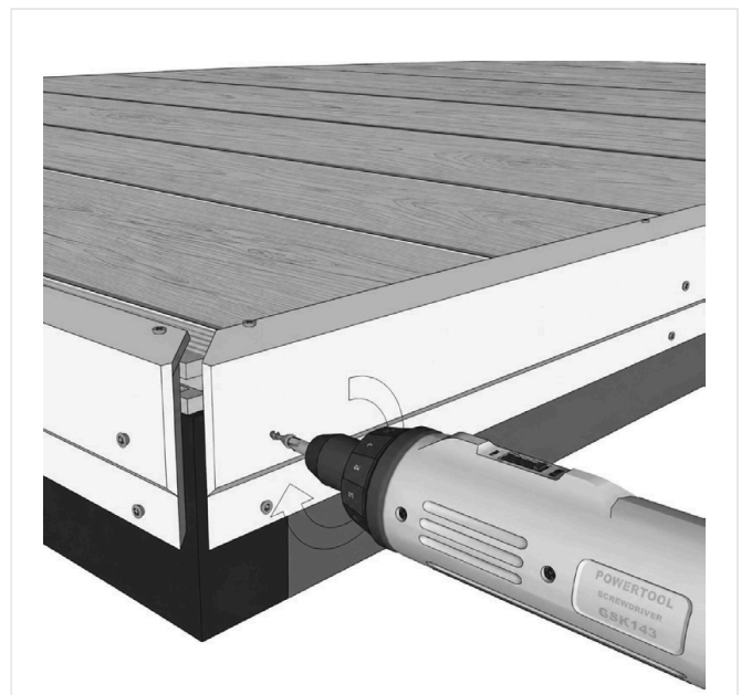
FIG. 26 - CORNER TRIM FIXED WITH COUNTERSUNK SCREWS
