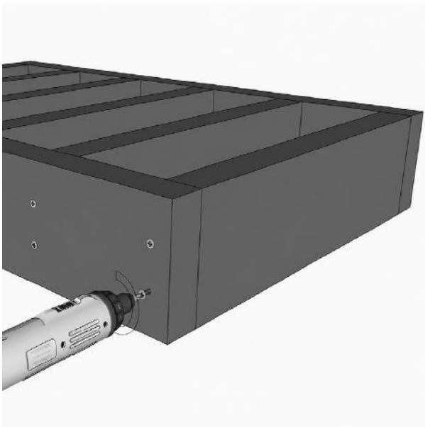
FIG. 27 – BOX FRAME BUILT TO SUPPORT THE STEP AREA
