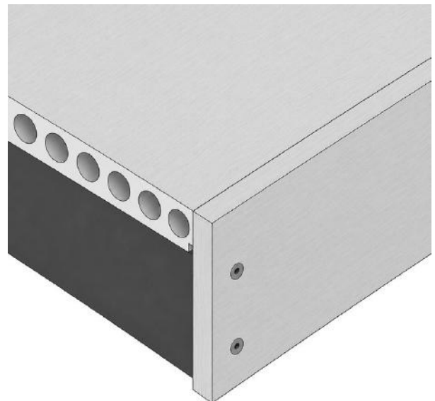
FIG. 24 – COUNTERSUNK PILOT HOLES PRE-DRILLED THROUGH THE FASCIA
