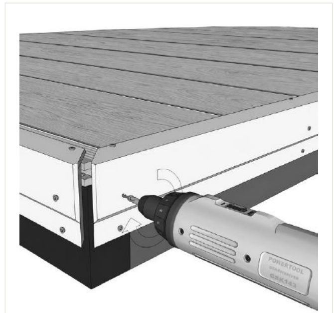
FIG. 26 – CORNER TRIM FIXED WITH COUNTERSUNK SCREWS
