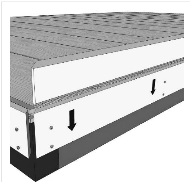
FIG. 25 – CORNER TRIM PLACED OVER THE DECK EDGE
