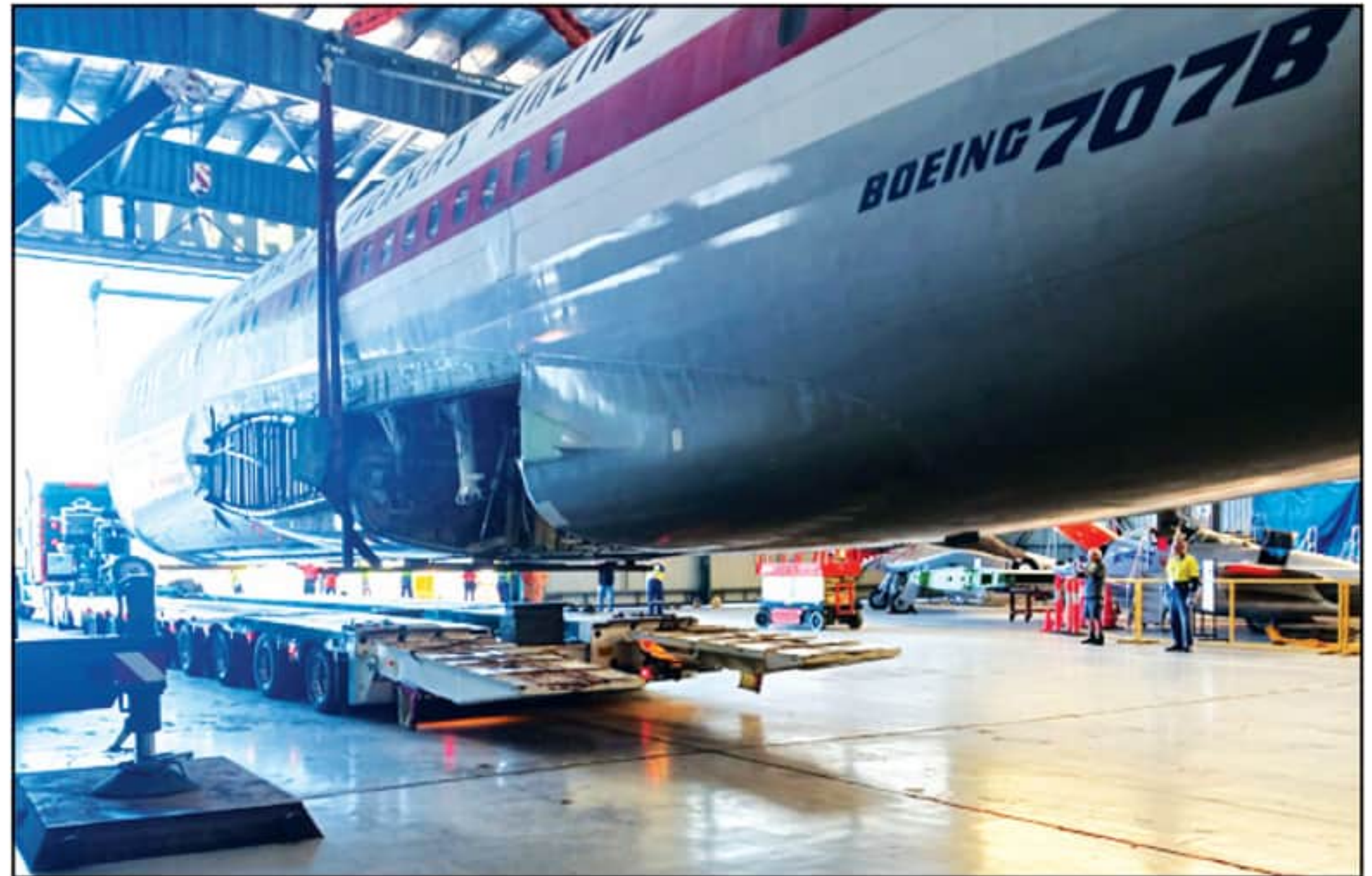
Lifting the aircraft off the trailer and setting it onto supports.
