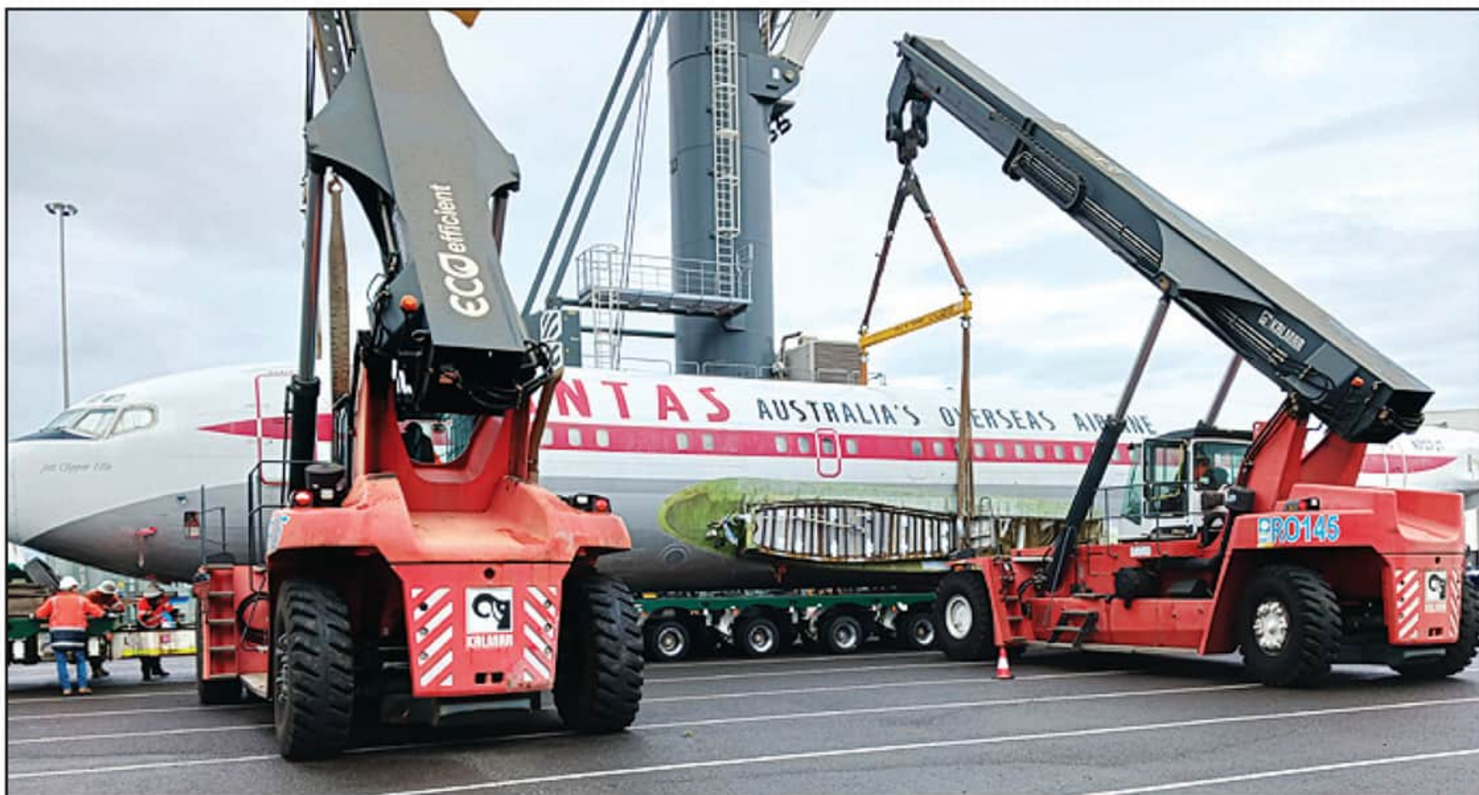
Lifting the fuselage onto the trailer for transporting to the airport.
