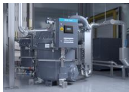
MDG dryer: A revolutionary heat-of-compression rotary drum desiccant dryer. It delivers a guaranteed, stable Pressure Dew Point (PDP) of -40°C with near zero power consumption.
