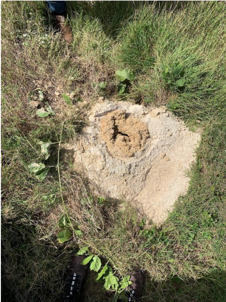
Image of the material extruded from the airtrack drilling process.
