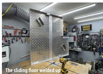
The sliding mechanism needs to be strong
