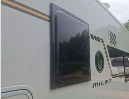
Washroom window sits proud
