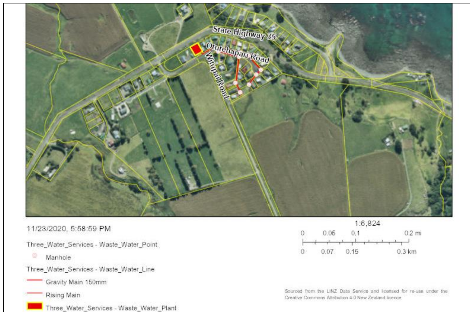
Figure 3 6 Wastewater network in Waihau Bay.
