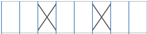
One cross brace every four bays
