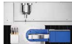
14 -Tool Automatic Changer Reduced manual intervention
