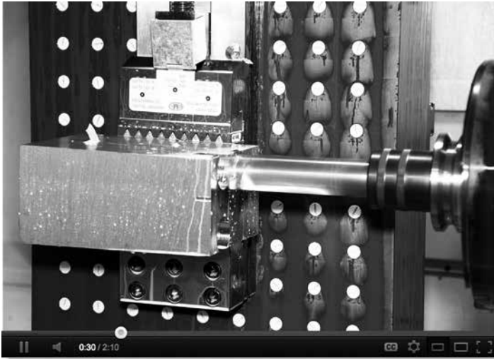
Milling on horizontal machining centre
