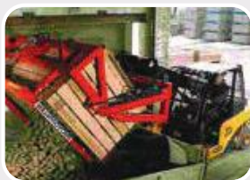
K80 forward tippler gentle & quick box tipping. Very adaptable & easy to operate
