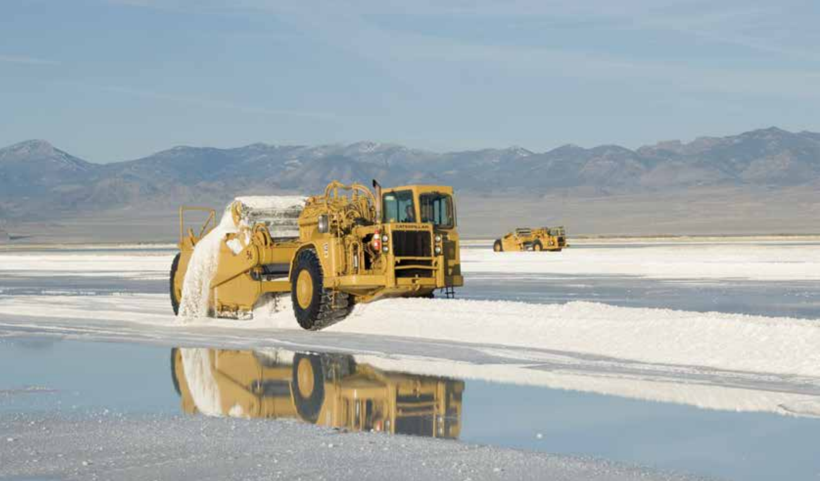
Harvesting at Intrepid's solar brine recovery mine in Wendover, Utah. After solar evaporation, mineral salts are collected from the ponds and processed to produce potash fertilizer.
