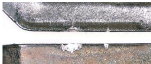
Chipping occurs at cutting length of 19.7 feet
