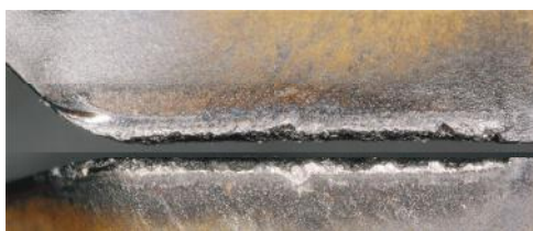
Chipping occurred due to peeling of the coating
