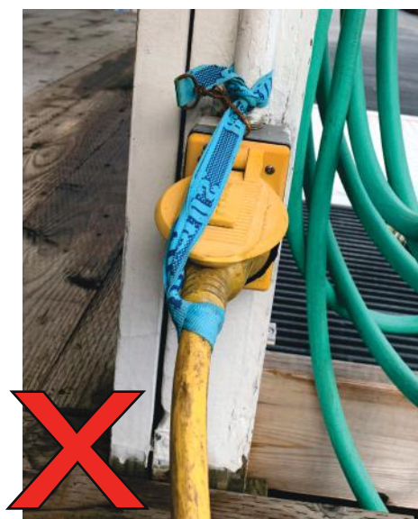
TWIST-TYPE INLET CHARRED FROM NORMAL USE
