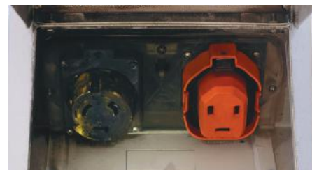
TWIST-TYPE INLET CHARRED FROM NORMAL USE
