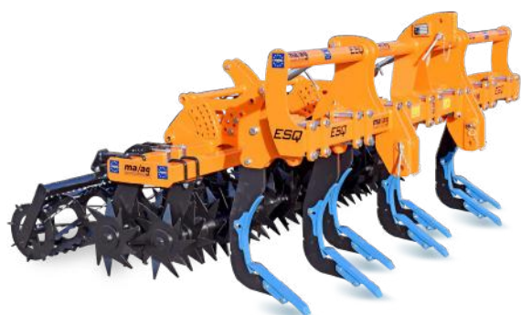
COMBINED EQUIPMENT FOR THE DOUBLE LAYER WORKING: DEEP TILLAGE AND SURFACE CRUMBLING ESQ AC
