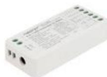
Sterownik do taśm / Controller for stripes LED COB 12-24V MIBOXER SR5 | IP20 | wymiary / size: 7,45 x 3,6 x 1,7 cm 005061 | EAN: 5907178025161
