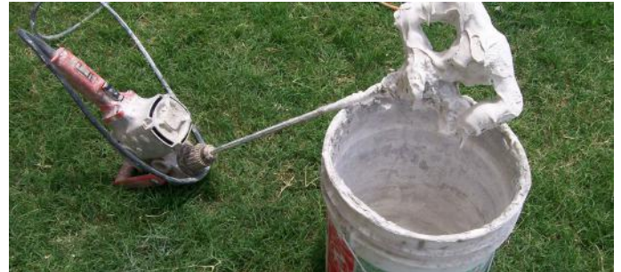
A thinset mixer requires constant cleaning. Always disconnect the mixer from the power source before cleaning.
