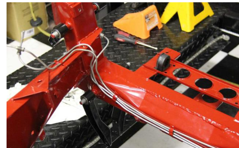
Extensive photographs were a big help in routing brake lines back the same way they were at the start.
