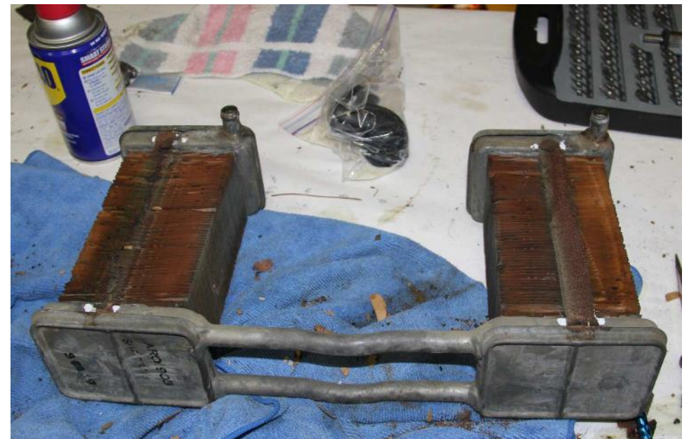
This is the heater core from the inside of the heater box. Once all the debris was cleaned out, the core pressure tested just fine, so back in it went. The outside of the heater box was bead blasted then painted with POR15 paint.
