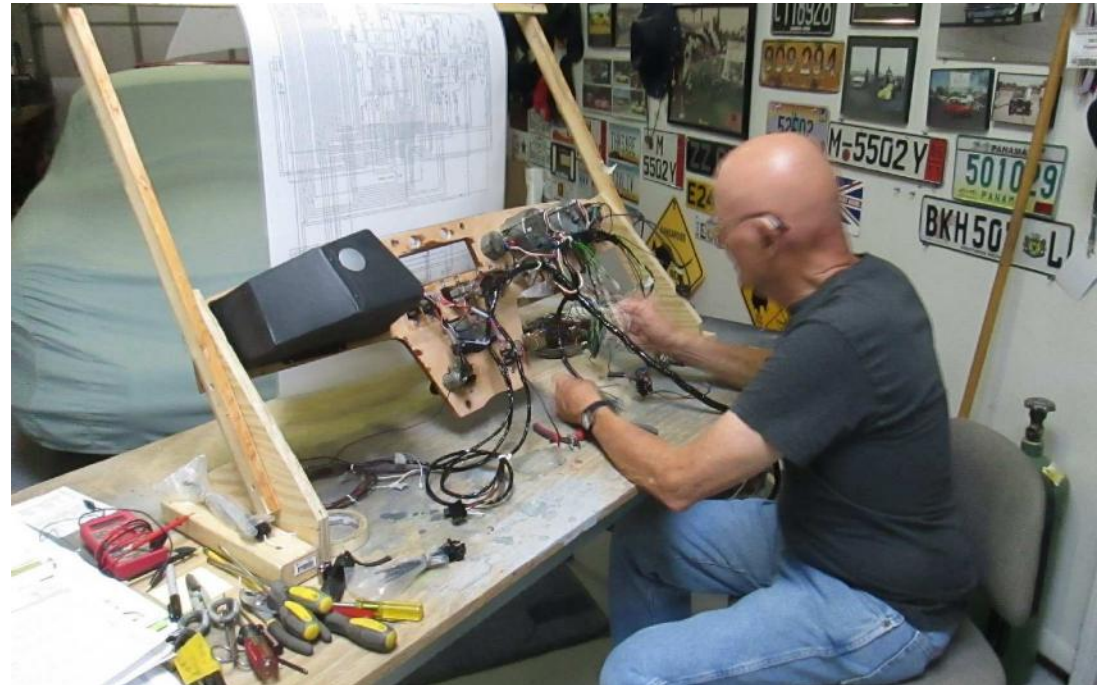
David Barnett built a frame to hold the dash and worked this project in his workshop. We took the original Lotus wiring diagram and blew it up and mounted it to a large, 4' X 5' poster board to help track down wires.
