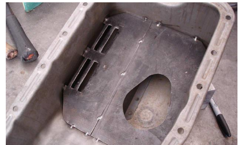
Duffee motorsports builds an oil pan baffle/windage tray that will reduce frothing in the oil pan and ensure the Elan always will have enough oil.
