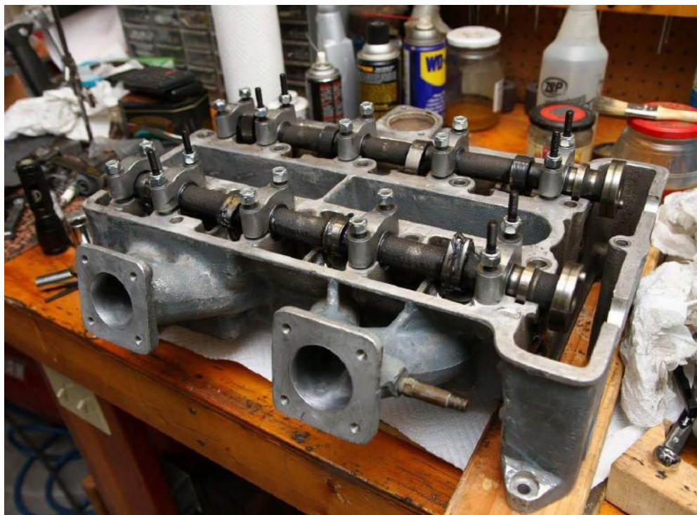
Cams installed with new bearings and valve lash set. Dave Bean's thin top tappets were used on the intake side to compensate for the 0.030" longer Sprint valves used. All hardware was cleaned. Caps for the crossover were reshaped and painted. All threads were chased.
