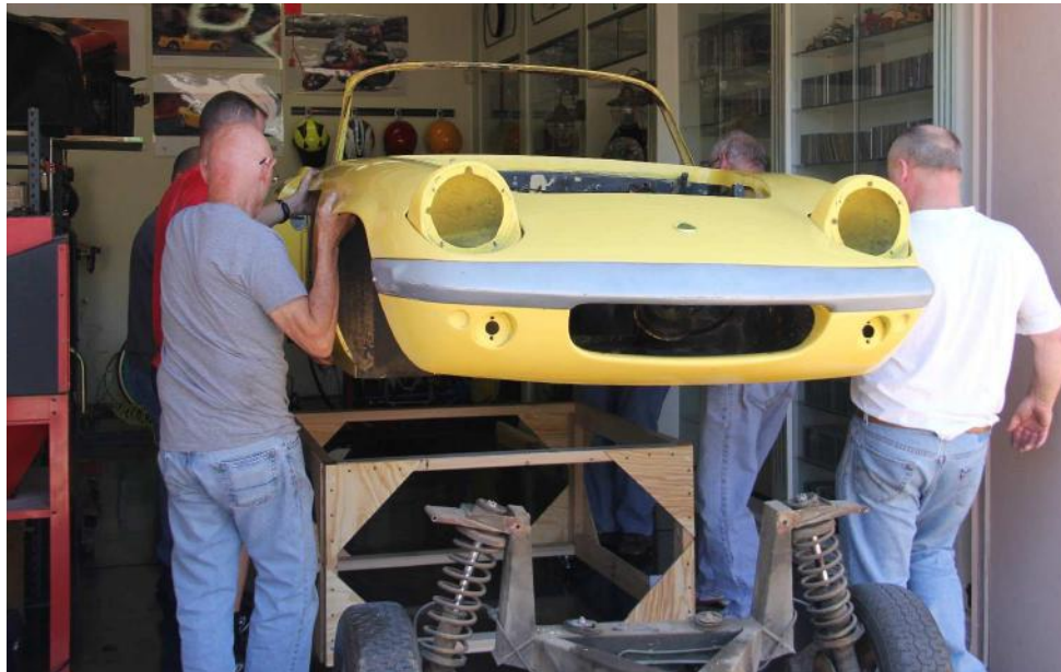
With enough guys gentling lifting and others searching around to find what was still sticking, the 220 lb. body quickly comes off. We carry it back into the garage and bolt it to Brett's custom made ingenious wooden frame structure.
