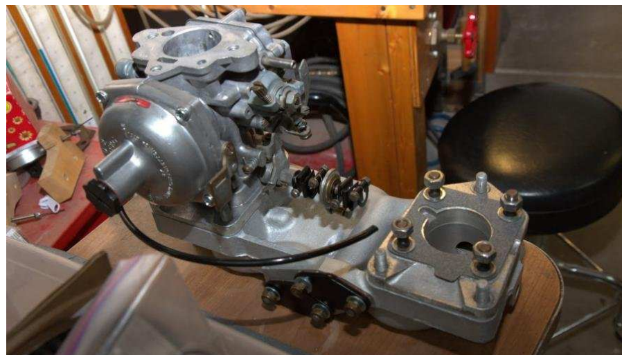
Each carb was rebuilt, preserving the original emissions stickers.
