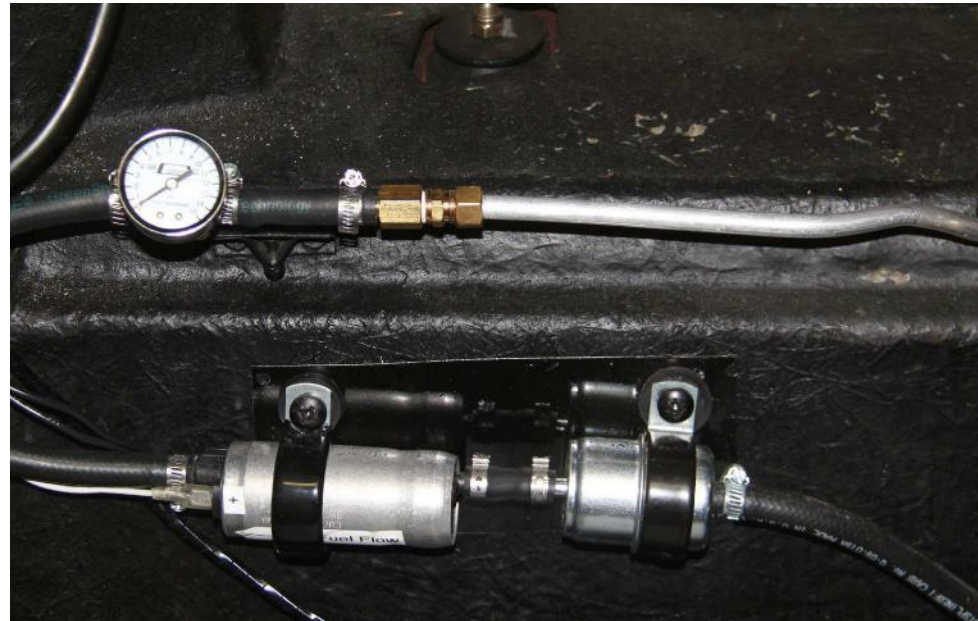
A new, reliable electronic fuel pump and filter are installed in the trunk, replacing the old mechanical pump. We also installed a fuel pressure gauge to get accurate data.
