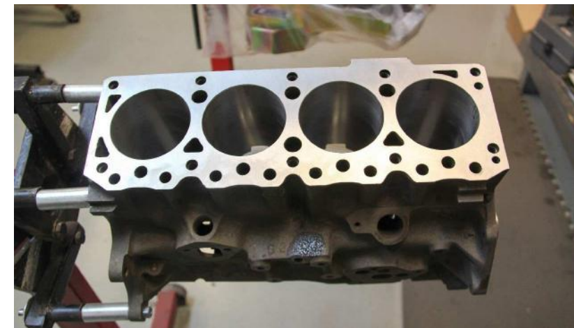
The original block is inspected, measured and then goes into the vat for cleaning. Then it's "decked" to insure it is perfectly true.
