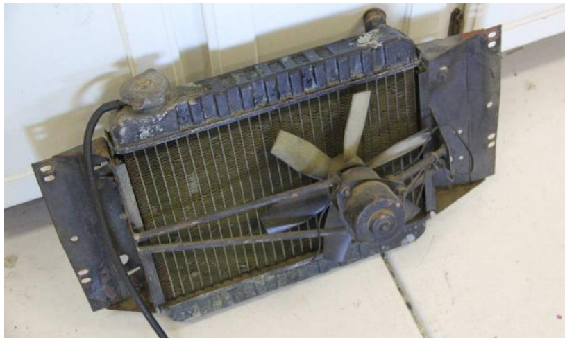
Here’s the old radiator. The new one provides over 4-5 times the cooling capability – and that’s without the new high powered fans.
