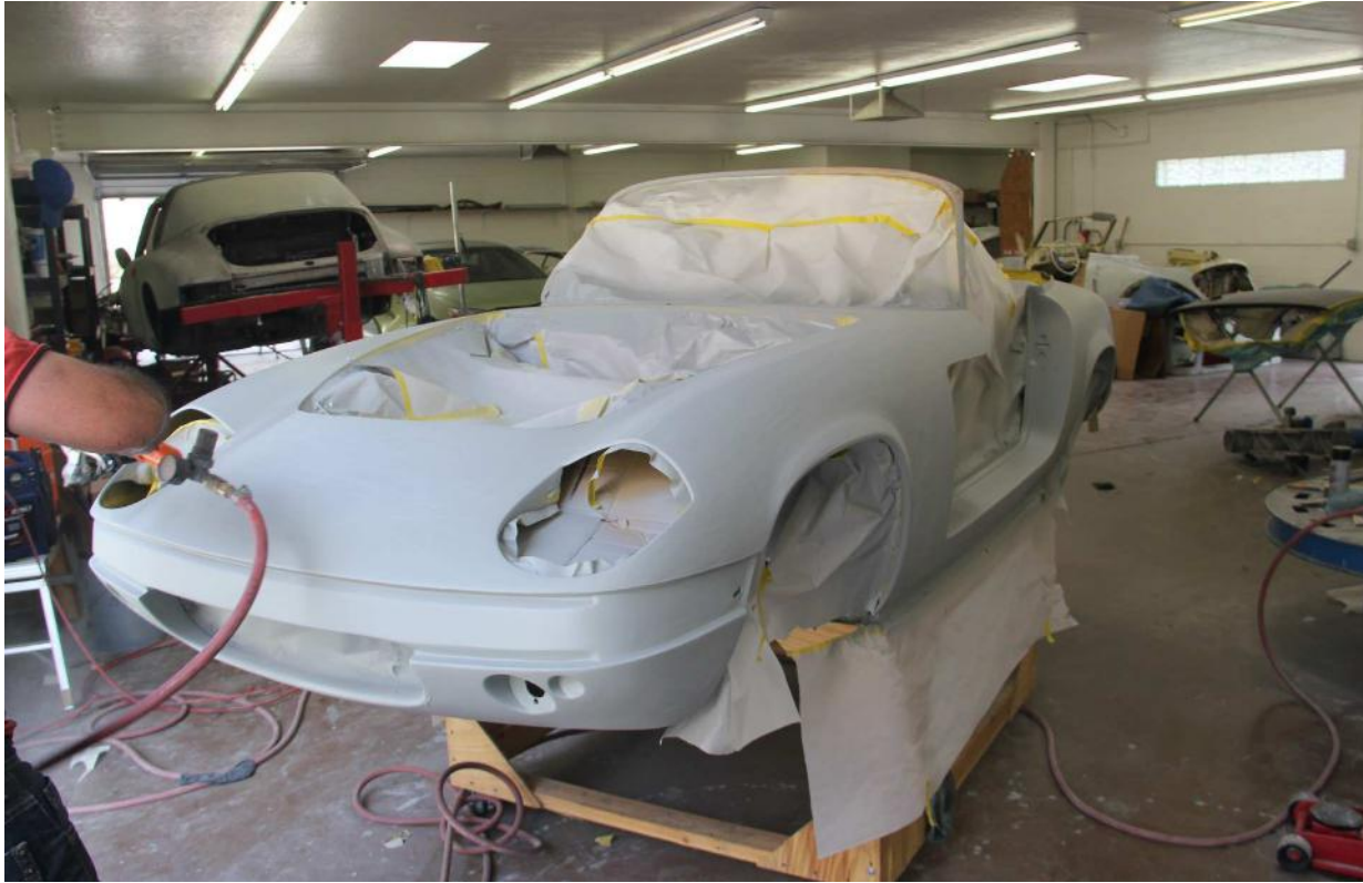
Top: Once all the old paint is removed and the body is perfect it is sprayed with “Kitty Hair,” a long strand fiberglass reinforced body filler. Bottom: After application of the fiberglass kitty hair and before the primer coat.
