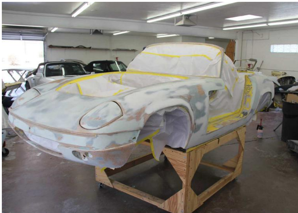
Before applying something called "kitty hair," we added fiberglass to several areas including the trunk and fiber-glassed in new bobbins.
