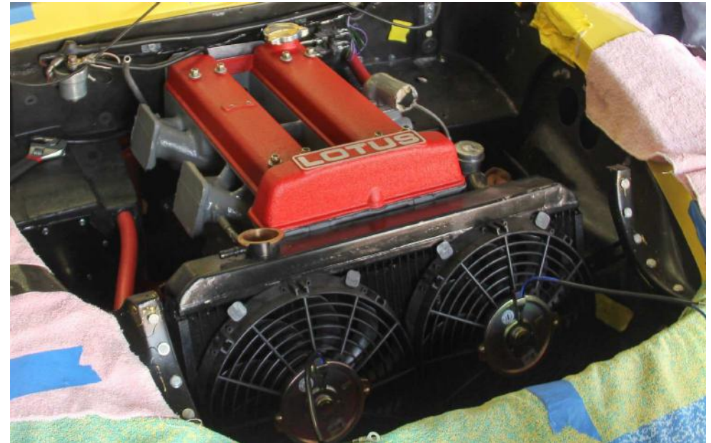
Today's technology allowed us to add two high performance fans, sealed to the front with more than enough juice from the Nippondenso alternator to power them. It was easy to reverse them into pusher fans.
