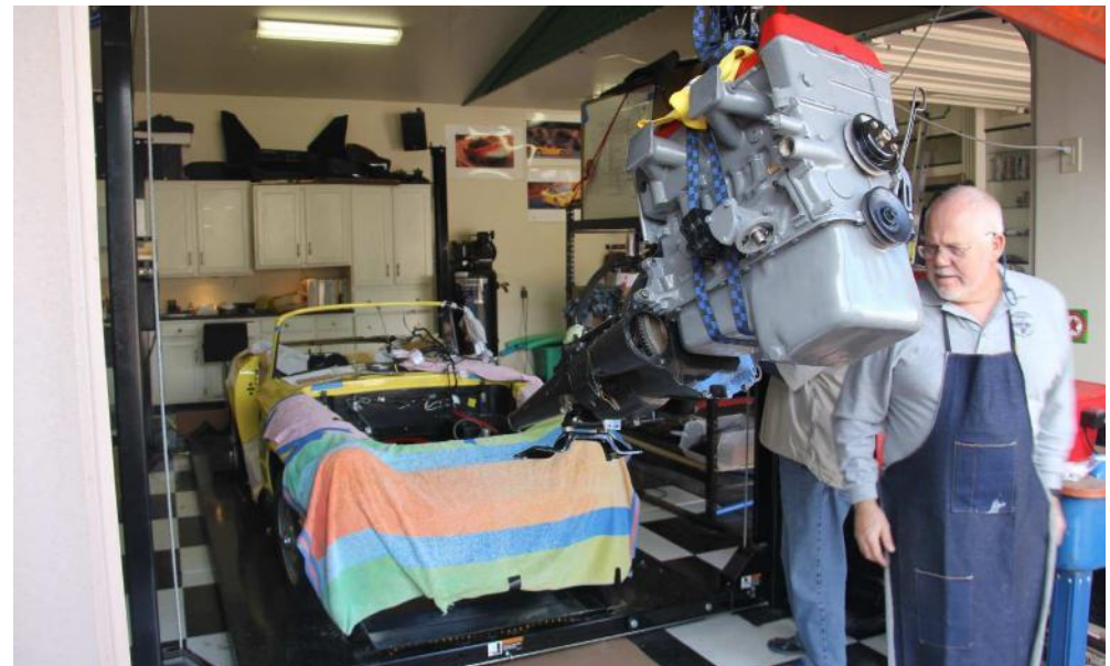
The completed engine, freshly back from Duffee Motorsports, is attached to the transmission. The two are put on the hoist to slide it back into the car. The towels are there not because the Elan is going to the beach, but to protect the paint.
