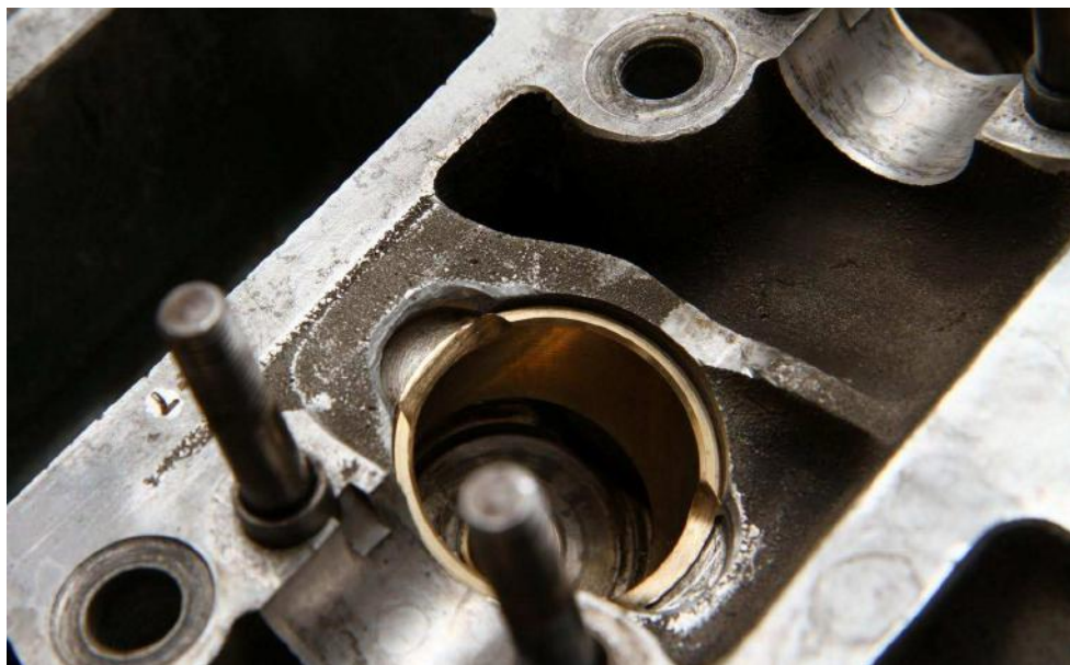
Bronze tappet liners were installed on the exhaust side.
