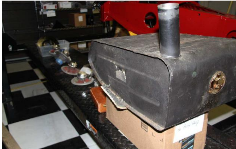
Gas tank “refurb” is straight forward. First, ensure not rust inside or out. Repaint exterior with POR15 and test and reinstall the sending unit with new gaskets.
