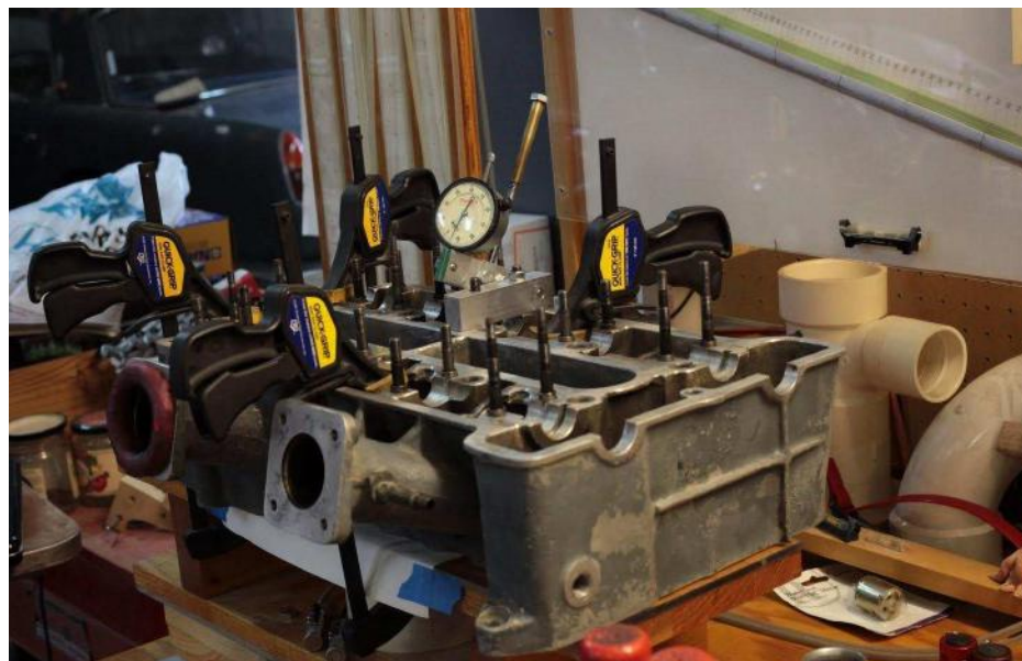
The Process: First the Elan head was flow tested in baseline condition (combustion chamber and valves decoked first). Then the carbs were installed and baseline testing was repeated. Testing established where the most gains were likely to occur.
