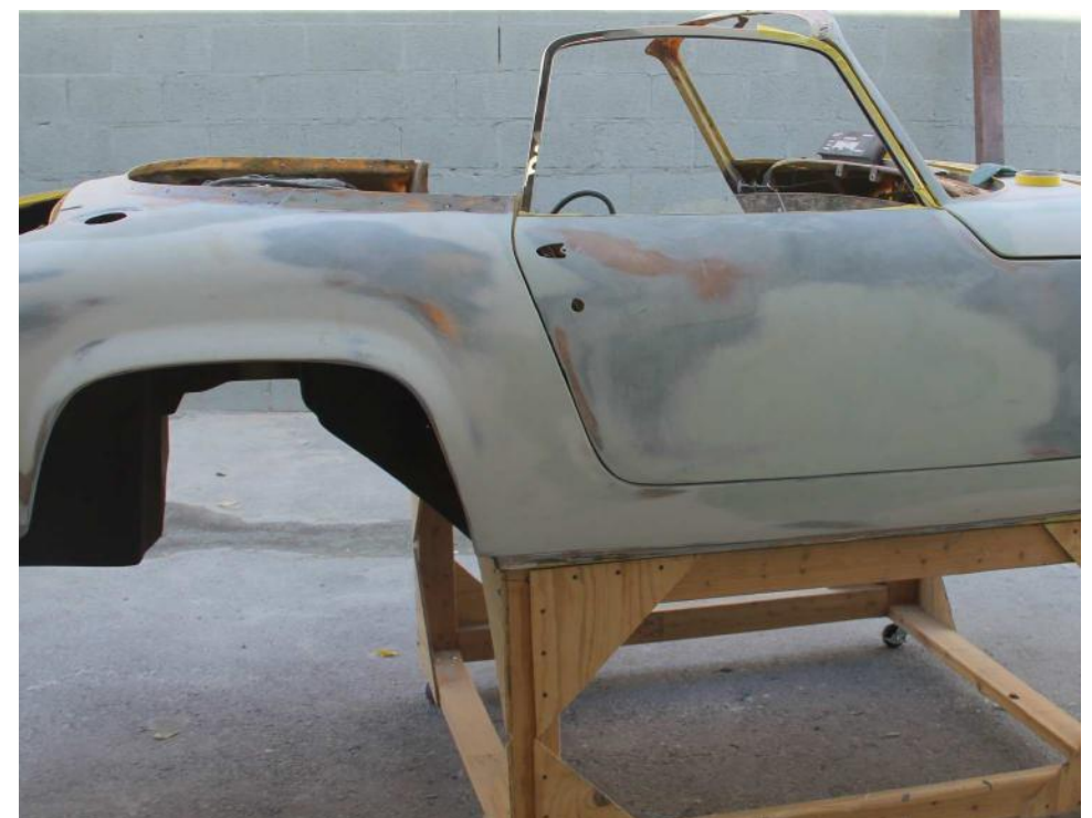
One noticeable flaw in nearly all Elans is ill-fitting, sagging doors. Some insist that originality requires leaving them this way. We elected to invest in the substantial effort to make them fit, no easy task. Here you can see the perfect fit, even before the car is painted.
