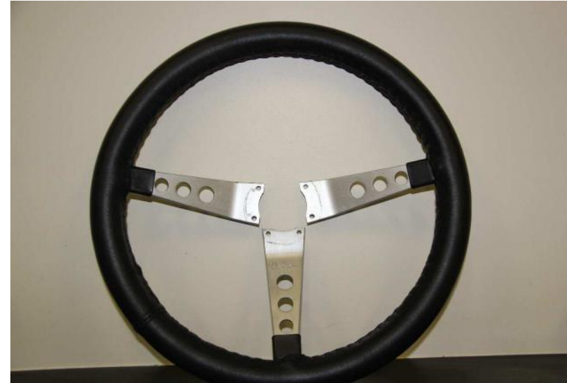
The original, Colin Chapman engraved steering wheel was in great shape. A heater hose and new leather cover makes it much thicker and like new.
