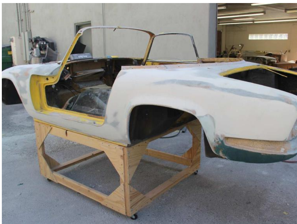
Based on Buckland recommendations, Kullukian reinforced areas of the body. The area holding the windshield got extra fill. Sometimes people reach for the windshield and use it to pull themselves out of the car – a really bad idea. Although not a problem on my car, it was smart to strengthen here.
