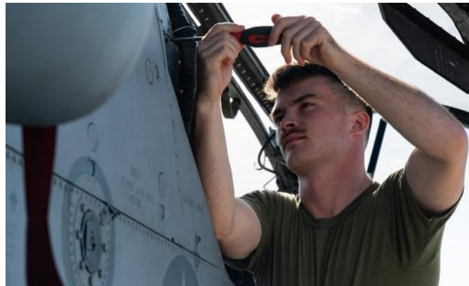
U.S. Marine Corps Sgt. Luke Tomasovitch, Marine Light Attack Helicopter Squadron (HMLA) 773 collateral duty quality assurance representative, loosens screws on an AH-1Z Viper helicopter control panel at Joint Base McGuire-Dix-Lakehurst, N.J., Oct. 2, 2026. Maintainers serviced the squadron's helicopters to ensure mission continuity and rapid response capability. (U.S. Air Force photo by Airman 1st Class Haeleigh Bayle)
