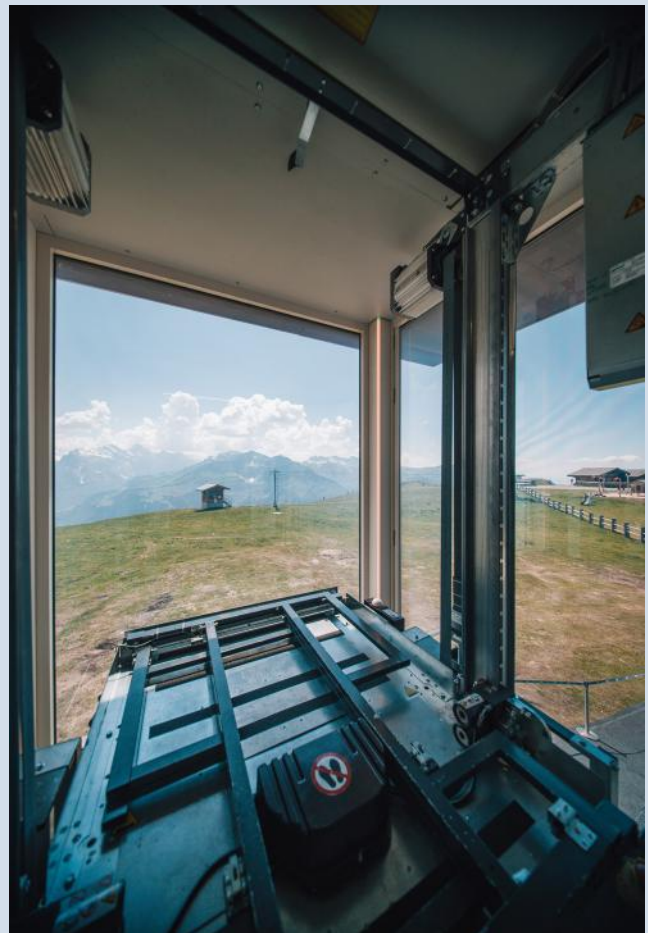
The car and two counterweights run on two rails.
