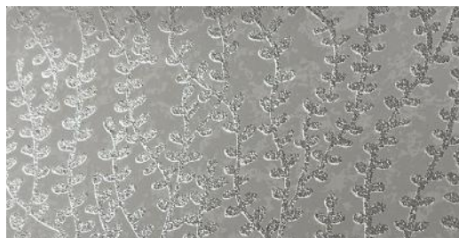
Print Style: Glass Beading Application Ink: Clear Adhesive Base Substrate: Non-Woven Paper
