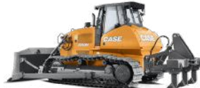
Dozers 20 Tonne 3D GPS/ Pat Blade Rippers
