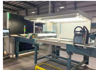
The Qualitron machine provides automated visual inspection of fired tiles, with the ability to detect defects, assess shade and tone, and ensure the design is in proper register.
