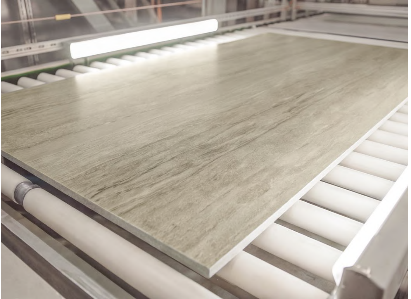
EcoStone porcelain panel on the MILE®stone production line. The line offers cross-cut and vein-cut aesthetics.
