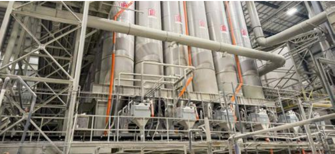
At Wonder Porcelain in Lebanon, Tenn., raw materials are wet-ground into liquid slip. This slip is then spray-dried into fine powder and stored in automated silos that provide a continuous feed of material to the press.
