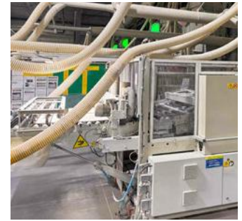
Using heat and pressure, the powder is converted into the unfired tile body.
