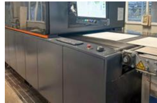
Designs and patterns are added to the body via an inkjet printer.
