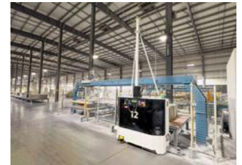
Automated guided vehicles (AGV) transport tiles and slabs in the factory, and RoboFloor, developed by System Ceramics in Italy, automatically handles, loads, and unloads fired tiles and large panels or slabs.
