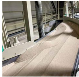
Conveyors deliver the powder to the press at Wonder Porcelain.
