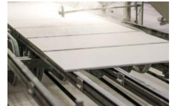
The tile body then travels through the glazing line.
