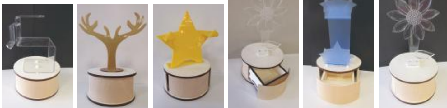
Small storage unit involving flexi-ply, vacuum bagging, CAD, Laser and vinyl cutting
