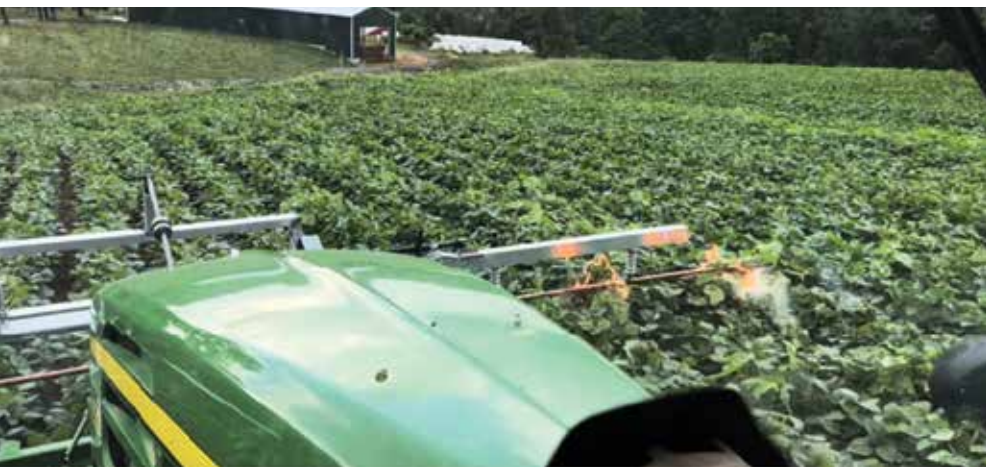
Lightning Weeder is a commercial tractor-mounted electric weed control unit that is currently being used in the U.S. to target tall weeds without the use of herbicides
