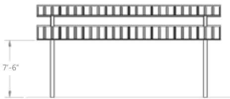
Minimum Clearance Height w/ MR Roof
