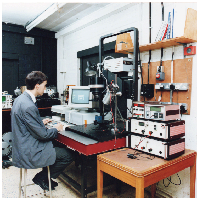
Peter at work in the optics lab (photo taken for publicity purposes). Equipment is for measuring the brightness and NVG-compatibility of cockpit displays. (1991)
