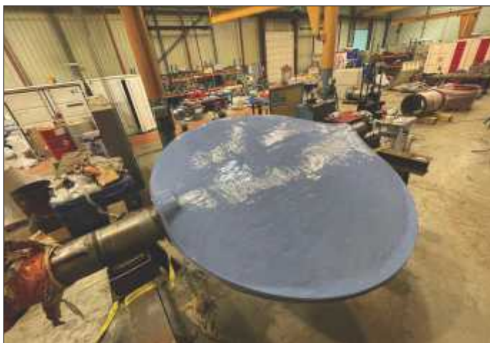
Lens of hydraulic valve coated with epoxy coating, Belzona 1341 (Supermetalglide).
