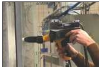
RoboTwin uses sensors to record the movement paths, recognizes the spraying process, and automatically generates an executable robot program for all common manufacturers.
