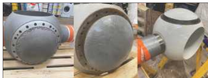
Damaged hydraulic ball valve repaired with Belzona 1000 Series systems.
