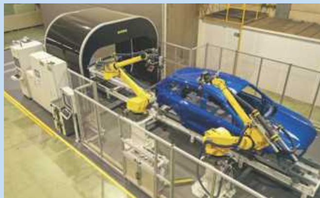
The ESFI system uses advanced AI algorithms and high-resolution optical technologies to precisely detect, classify, and locate surface defects such as dust inclusions, craters, runs, or scratches – directly on the production line and without stopping production.
