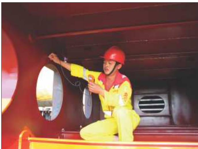
Technical service engineer conducting coating thickness measurement and inspections to ensure compliance with protective coating specifications and durability requirements.
