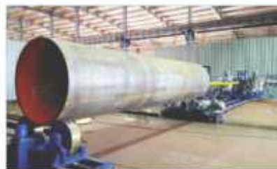
Internal Automatic Pipe Coating
