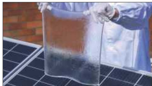
Findings from the PolyU research team showed that applying this hydrogel coating to solar panels could reduce hot-spot temperatures by up to 16°C and enhance power output by as much as 13%.
