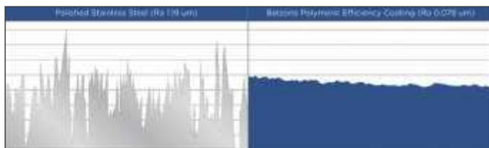
Roughness comparison between polished stainless steel and Belzona 1341 (Supermetalglide). Surface inspection: Leeds University.
