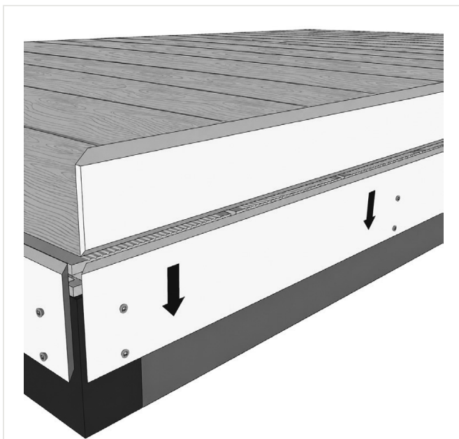
FIG. 25 - CORNER TRIM PLACED OVER THE DECK EDGE
