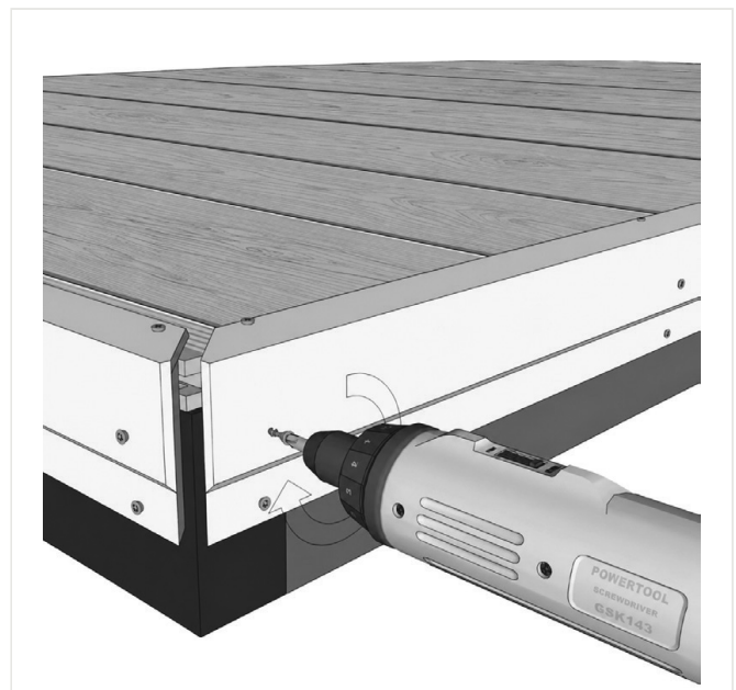
FIG. 26 - CORNER TRIM FIXED WITH COUNTERSUNK SCREWS
