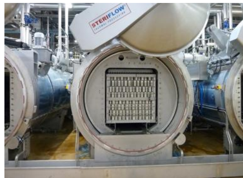
Rotary Steriflow diameter 1800mm
