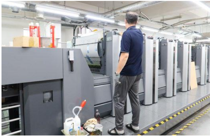
The LED-UV equipped RMGT 970PF-8 has enabled shorter lead times and eco-friendly printing
