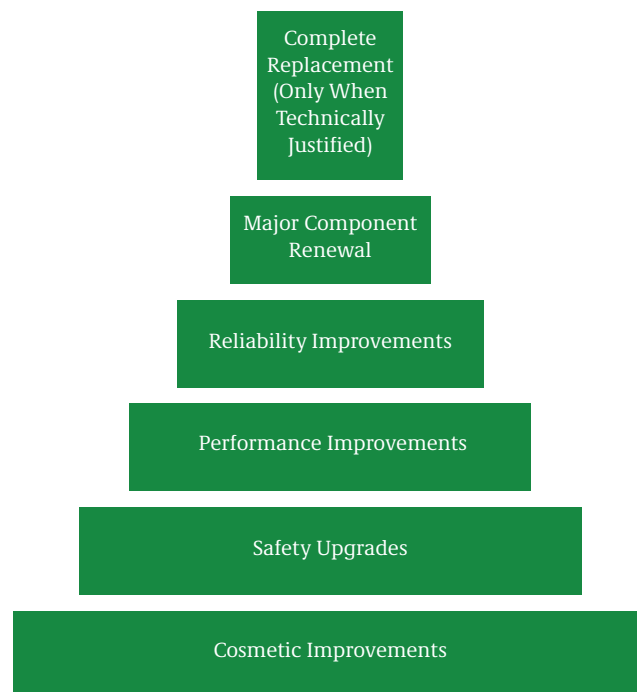
Figure 1: The Escalator Modernization Decision Pyramid proposed by your author illustrates a structured decision-making framework in which modernization progresses from cosmetic improvements to complete replacement based on engineering assessment and life-cycle considerations.
