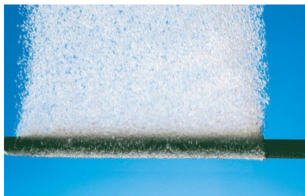
Microbubbles produced by sparger
