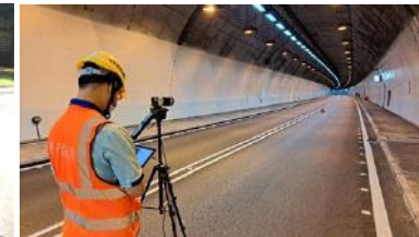
▲ Electrical Technology Center: Tunnel and Road Lighting Measurement
