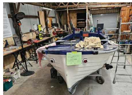
Renovation showing new paintwork, fixtures, fittings & rowlocks
