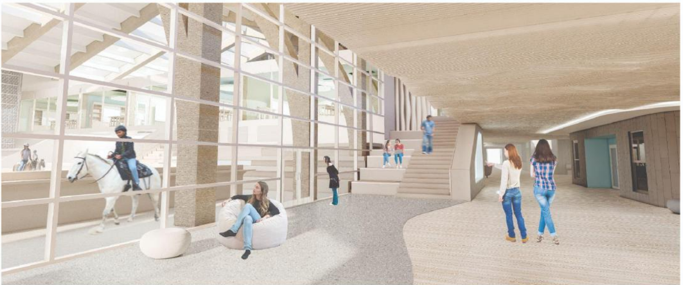
Fig. 18: Lobby entry, prioritizing analogous colors with low-contrast “pops” of color achieved by using wood, rubber vinyl flooring, acoustical ceiling baffles, diffused daylighting, and linear cove lighting.
