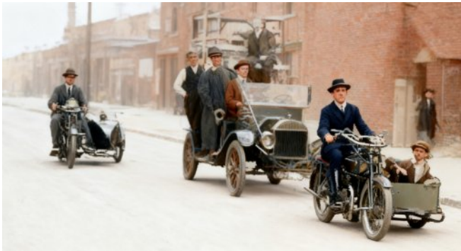
1916 Cont'd: "A sidecar towing a broken down light lorry carrying 5 cwt. of goods and five men. The machine is a single-cylinder 4hp Excelsior."
