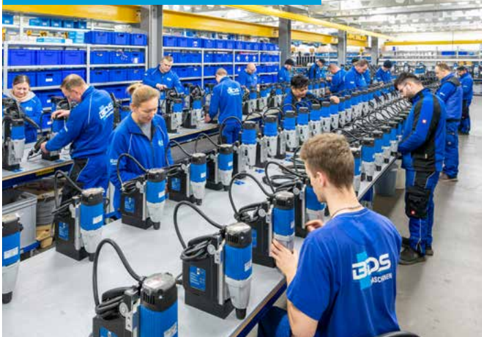
Assembly line for magnetic drilling machines
