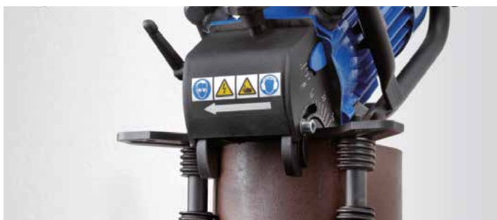
Edge processing of pipes in vertical position.
