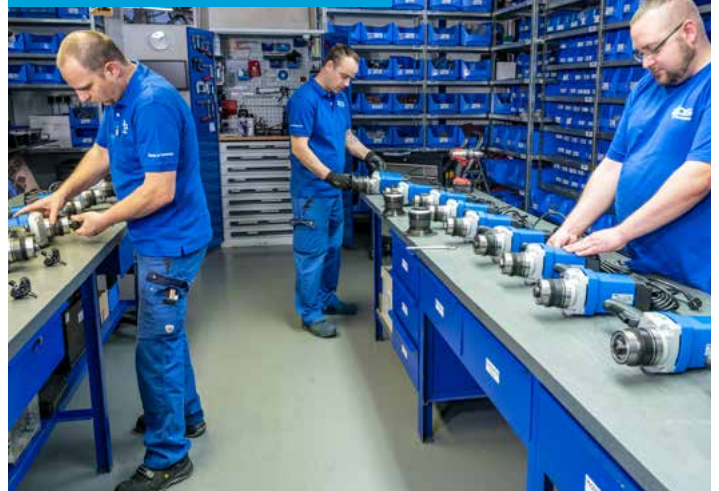
Assembly line for bevelling machines
