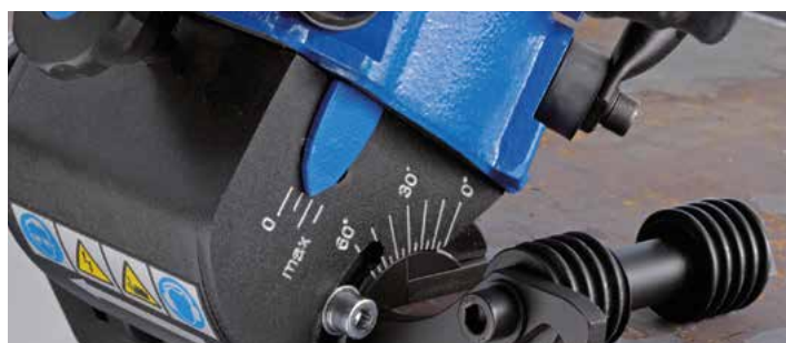
Continuous angle adjustment from 15° to 60°.
