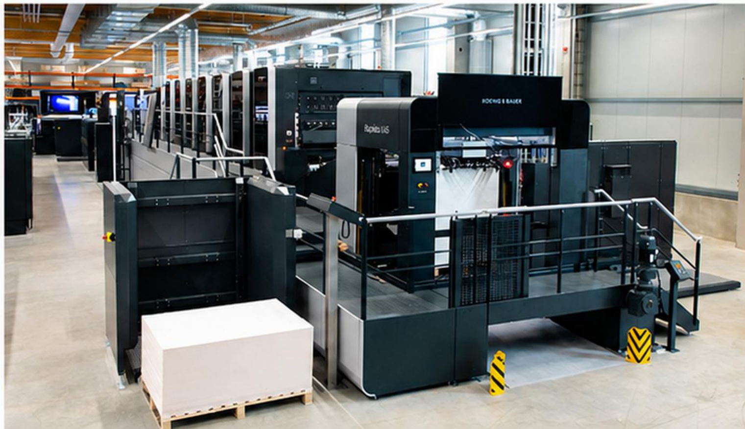
Photo 2: Rapida sheetfed offset presses, such as this Rapida 145, feature assistance systems like AutoRun, AutoSet, and JobGuide that execute set-up processes autonomously and standardise pressroom operations
