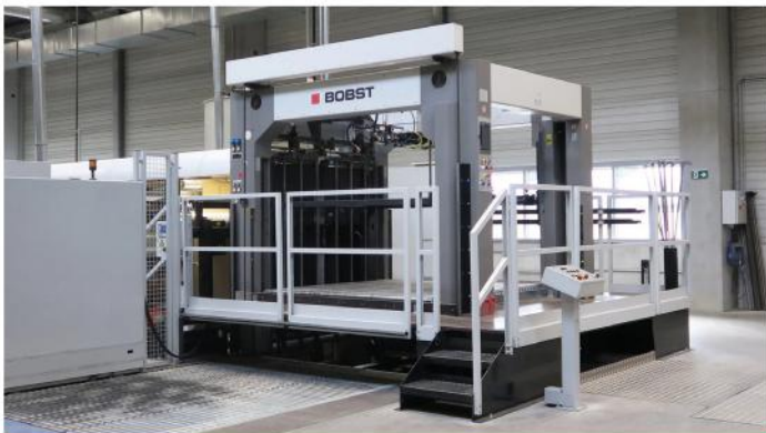
POWERALIGNER connects to the SMART FEEDER, enabling automatic correction of the stack position.
